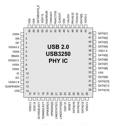
Figure 3.1 56 Pin USB3250 Pin Configuration (Top View)
