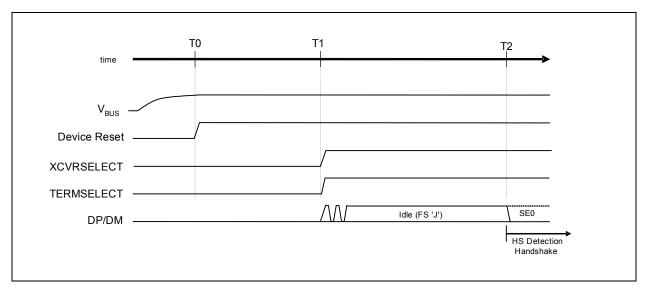
Figure 8.8 Device Attach Behavior
