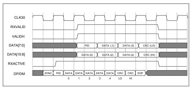
Figure 7.8 Receive Timing for 16-bit Data, Even Byte Count
