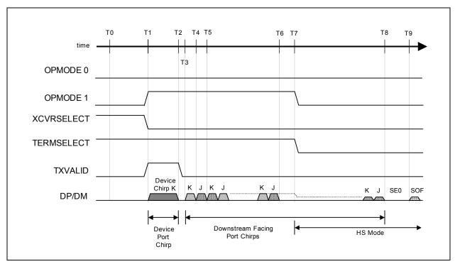
Figure 8.5 HS Detection Handshake Timing Behavior (HS Mode)
