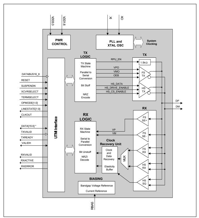
Figure 2.1 Block Diagram
