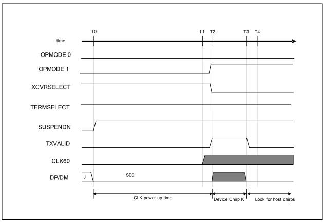
Figure 8.6 HS Detection Handshake Timing Behavior from Suspend
