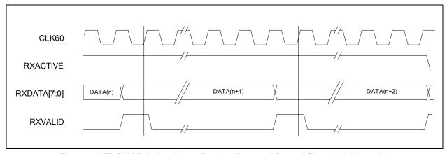
Figure 7.3 FS CLK Relationship to Receive Data and Control Signals (8-bit mode)
