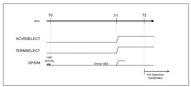
Figure 8.1 Reset Timing Behavior (HS Mode)
