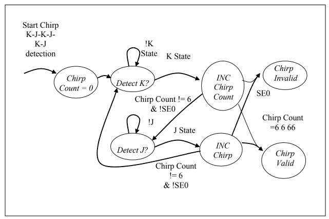
Figure 8.4 Chirp K-J-K-J Sequence Detection State Diagram
