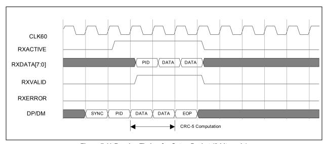
Figure 7.11 Receive Timing for Setup Packet (8-bit mode)
