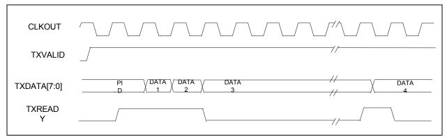
Figure 7.2 FS CLK Relationship to Transmit Data and Control Signals (8-bit mode)
