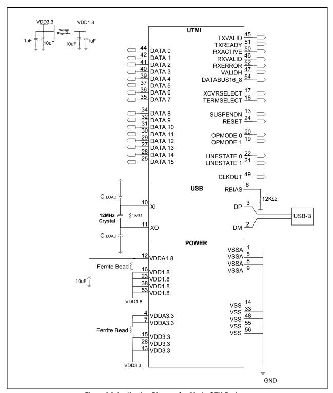
Figure 8.9 Application Diagram for 56-pin QFN Package
