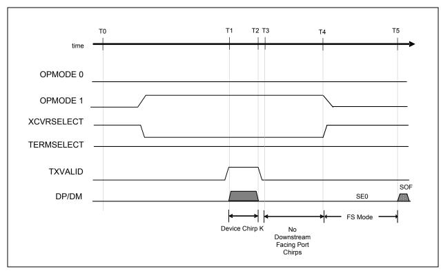
Figure 8.3 HS Detection Handshake Timing Behavior (FS Mode)
