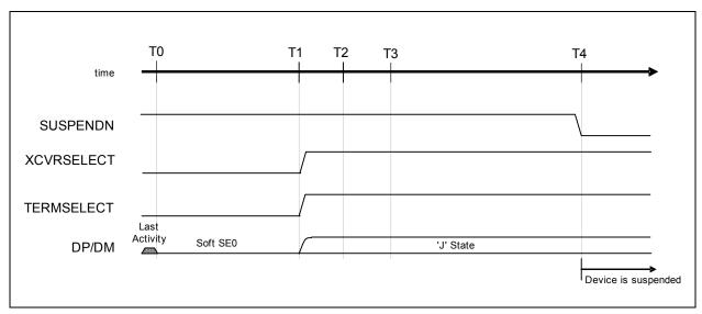
Figure 8.2 Suspend Timing Behavior (HS Mode)
