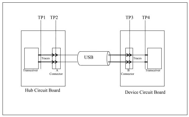
Figure 6.3 Eye Pattern Measurement Planes
