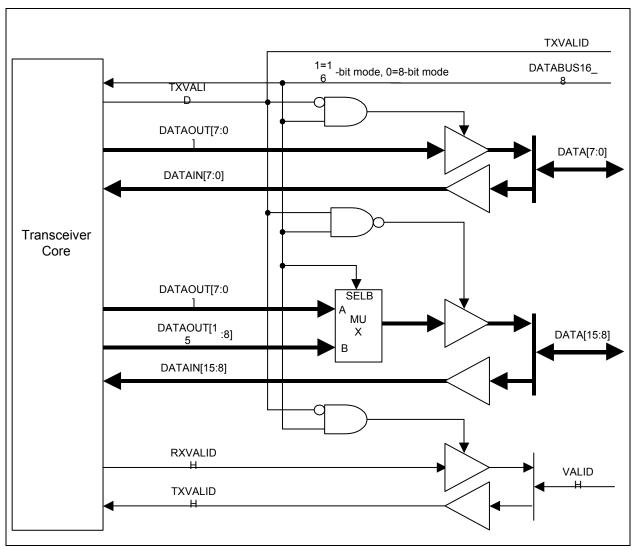
Figure 7.1 Bidirectional 16-bit interface
